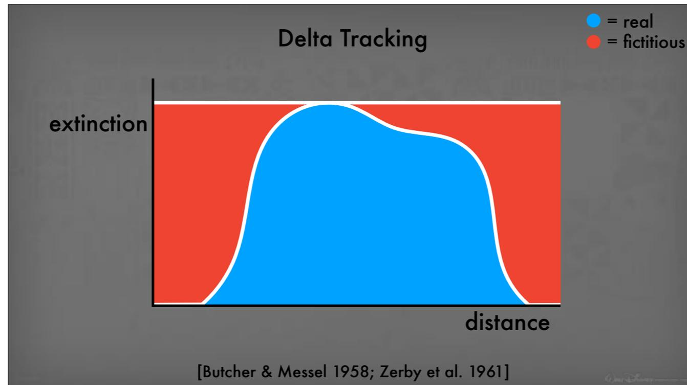
Here's a plot of the extinction along the ray. We take a step forward as if the volume were homogeneous with the maximum extinction coefficient of the combined volume, look up the ratio of real and fictitious media at the point, draw a random number, and check whether it corresponds to the real or fictitious medium. We repeat this process until we hit the real medium.
