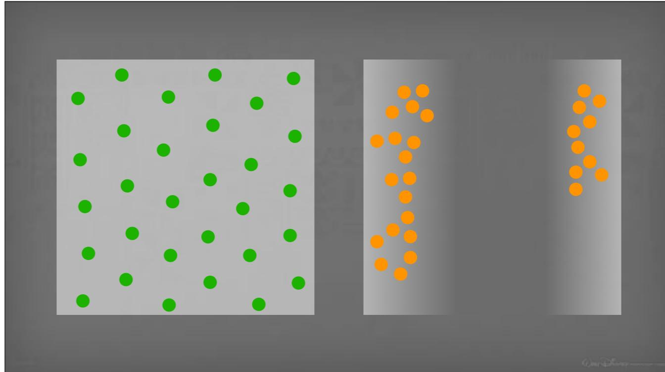
It turns out that we can, and this leads to the basic version of our decomposition tracking algorithm. We sample a separate distance in each component. Then to combine them into a single distance, we take the minimum of the two. As we prove in the paper, this produces the correct distribution of distances, the same distribution as delta tracking.
