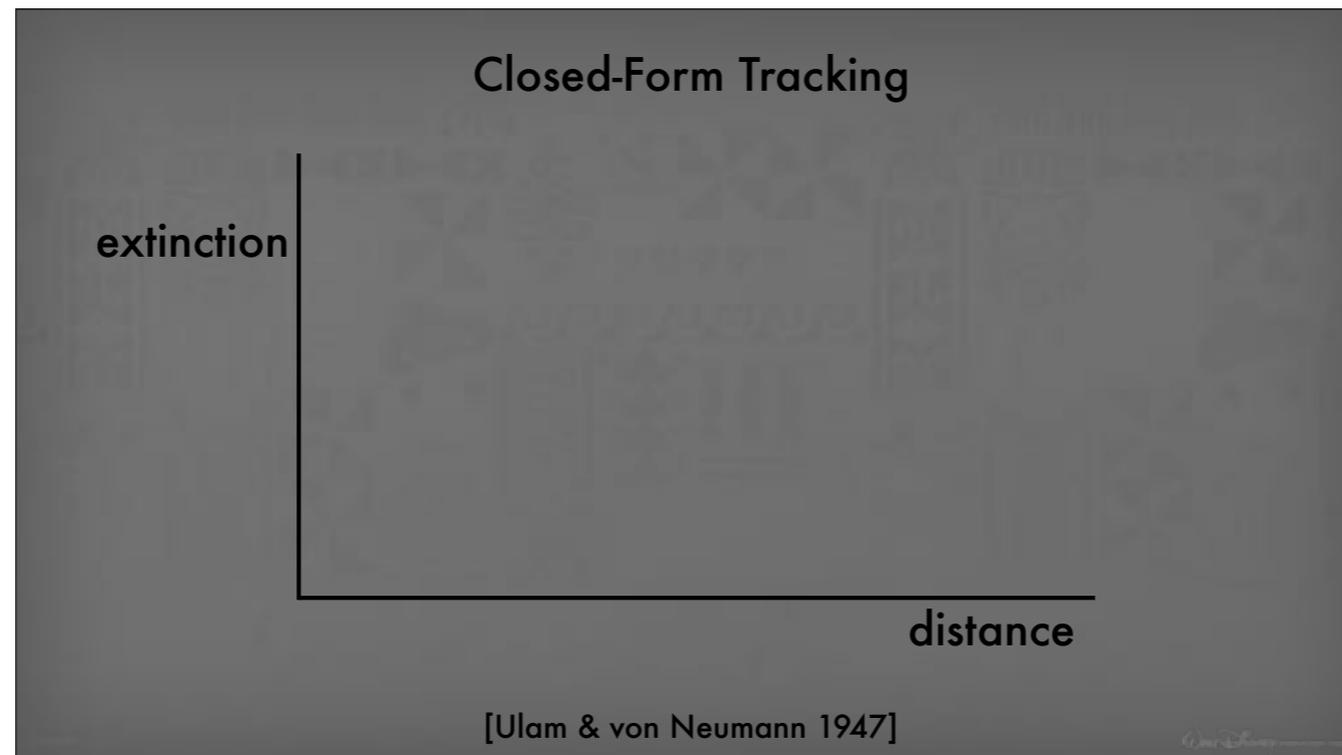
Here's a different view of the process for the slice of the volume along the ray, with the distance along the ray on the horizontal axis and the density, or, more precisely, the extinction coefficient, on the vertical axis. We simply sample a single distance from the exponential distribution and that tells us the scattering location.
