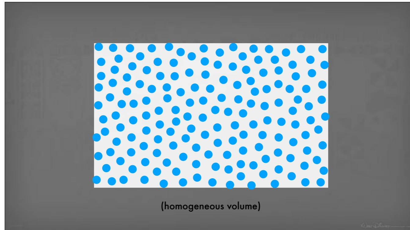
Here's a schematic 2D diagram of a rectangular volume, which can be thought of as being composed of particles. This happens to be a homogeneous volume, one with the same properties throughout. It has a uniform density.
