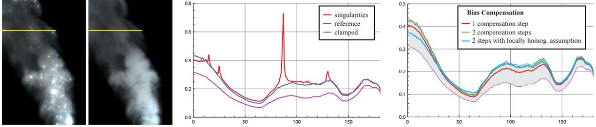
**Figure 4:** Left: we use the highlighted scanline to illustrate our observations. Center: plot of the pixels’ radiance when computing the image with un-clamped VPLs (exhibiting singularities, red), clamped VPLs (purple), and ground truth (full compensation, blue). Right: radiance plotted for ground truth and clamping (top and bottom boundary of the band), with 1 (red), 2 (green), or 2 locally homogeneous (blue) additional compensation steps.
