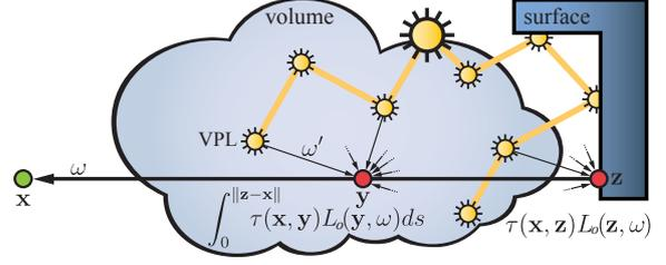
**Figure 3:** Light transport in participating media: radiance arriving at a point equals the sum of the integrated, in-scattered radiance and the radiance reflected off the surface. Indirect illumination and multiple scattering is computed by gathering from VPLs.
