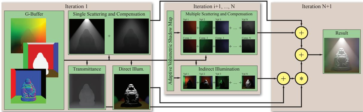
**Figure 9:** Data flow in our progressive GPU renderer. In the first iteration we compute the geometry buffer, single scattering with bias compensation from primary light sources, transmittance, and direct illumination. In each subsequent iteration we compute multiple scattering, indirect illumination, and bias compensation due to a single VPL, and add it to the final result.
