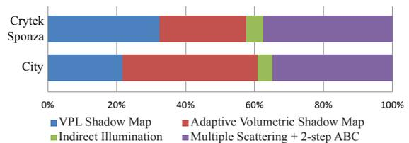
**Figure 10:** Shading time per VPL for the Crytek Sponza and City scenes: most of the shading time is used for constructing the shadow maps (about 60%), while indirect (surface) illumination is relatively fast, and multiple scattering with 2-step ABC requires only 35 – 38% of the entire shading cost.
