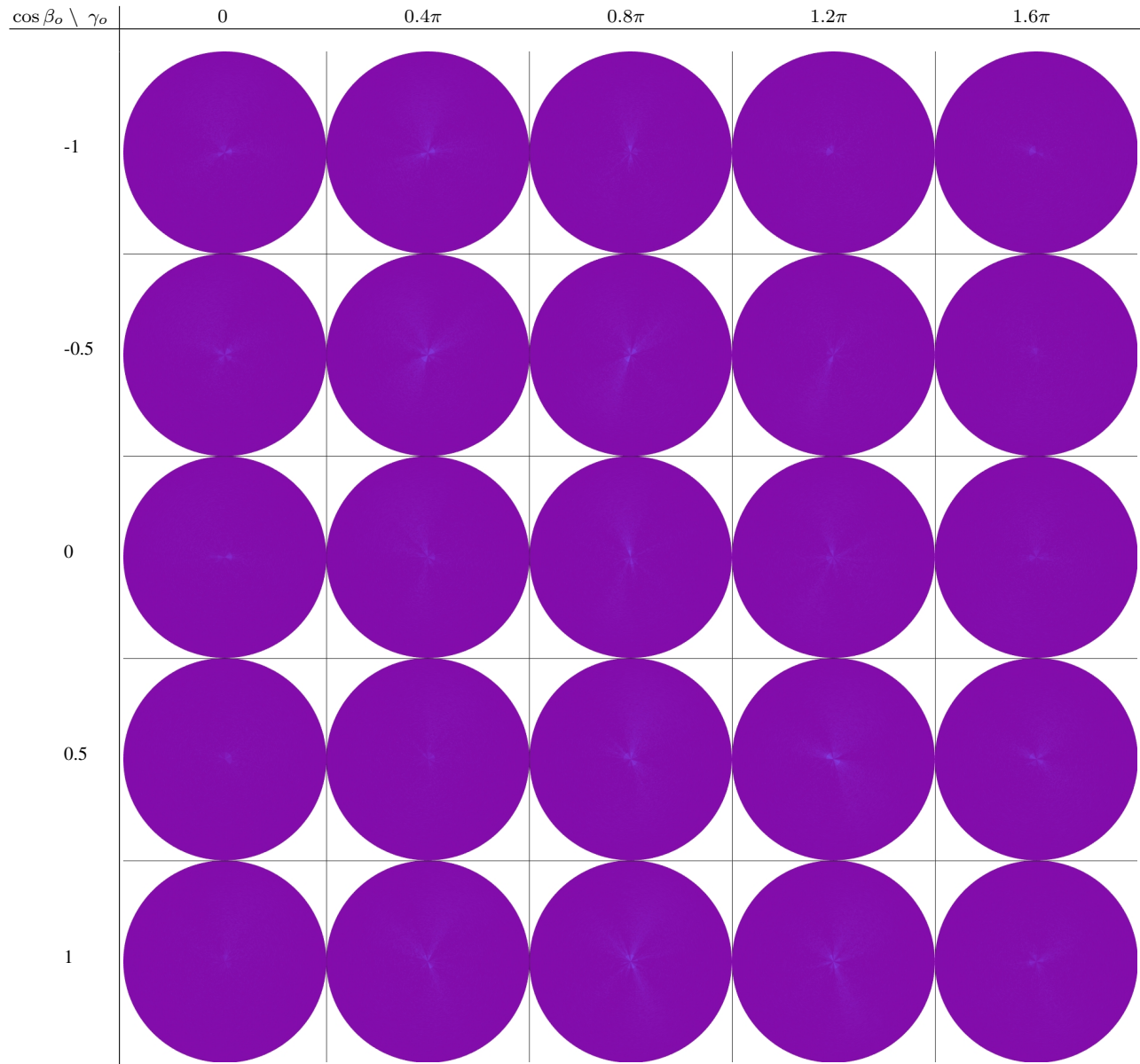
Figure 25: Front-facing directional GSDF approximation error e_{f_g}(\vec{\omega}_i, \vec{\omega}_o) on hairball grains. We visualize this 4-dimensional error function by plotting slices through \cos \beta_o (vertical) and \gamma_o (horizontal). The individual circular heatmaps encode \sin \beta_i as the distance from their center and \gamma_i as their rotational component.
